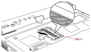
Figure 3-11 Installing the memory module
